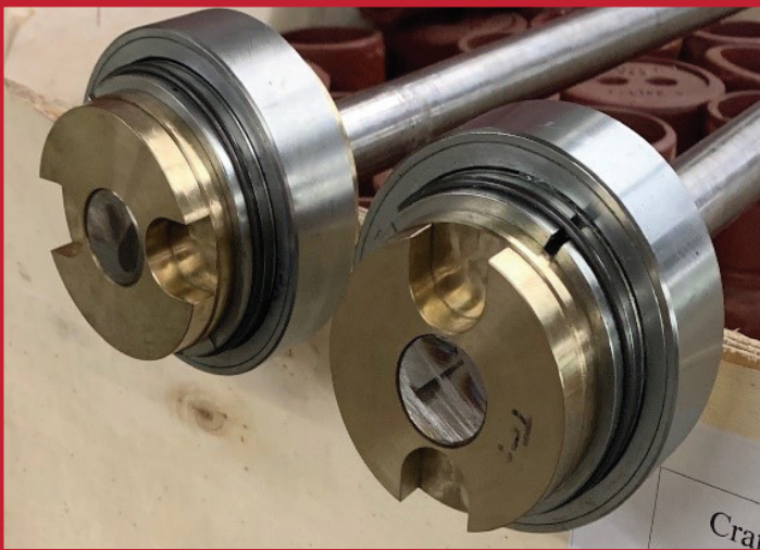
Drive nuts machined for electric actuators
