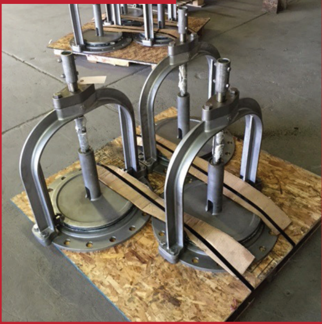
16 inch cast 316 stainless steel mud valves ready for deliver
